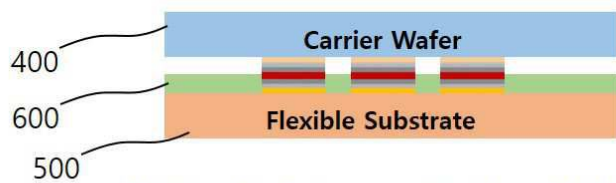
Chip Transfer/Interconnection through ACF Bonding (ACF 본딩을 이용한 LED 칩 전사/접속)
